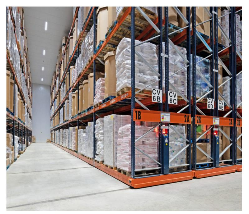
mously. This is the only compact system that provides direct access to the goods. It does so by opening the required aisle by means of a remote control or directly via the onboard control panel.
