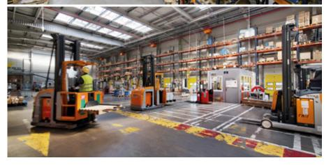
As a safety measure, racking uprights have been protected to absorb possible impacts produced by the handling equipment while manoeuvring unit loads.
