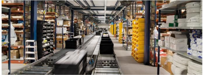
Racking levels are made out of perforated shelves that, in addition to having a high load capacity, favour the flow of water in case the fire safety system is activated. Furthermore, vertical side meshing has been attached to the ends of the racks.
