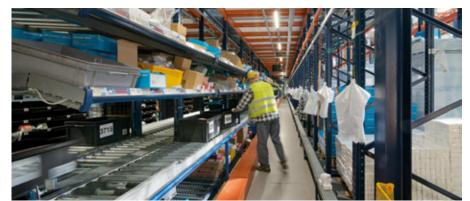
The picking block consists of live storage racks for pallets and boxes, racks with shelves and a conveyor circuit that creates two order prep areas on each floor
