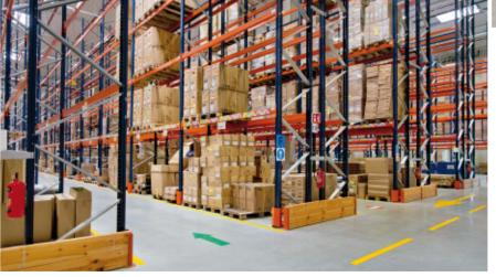
Decathlon, the established sports equipment chain, has constructed a new 30,000 m² logistics centre in Łódź (Poland) and Mecalux has fitted it out with picking shelves and pallet racks. Both solutions help classify the goods according to their dimensions and demand, while also providing direct access to speed up order picking, this centre's primary operation.
