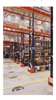
The racks allocated to picking stand an impressive 9.5 m high. One of their interesting features is that pick shelves are located only 3 m below, while palletised reserve products are set in the 6.5 m above. As such, needed goods are always available and picking runs uninterrupted.
