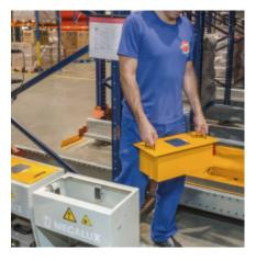
The operator sends movement orders to the Pallet Shuttle by means of a Wi-Fi connected tablet. It has a touch-screen interface and a very intuitive software that requires no special training to use. Each tablet can interact with all the shuttles in the warehouse, following a prioritisation protocol. The battery charging system is easily accessible to operators. A spare insertable battery means the shuttles are always operational.
