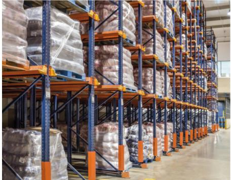
Operators, pushing reach trucks, enter the inner lanes with the load raised above the level where it is going to be deposited. On the floor, guide rails make it easier for forklifts to be centred and move safely inside lanes, minimising accidental damage to the racking.
