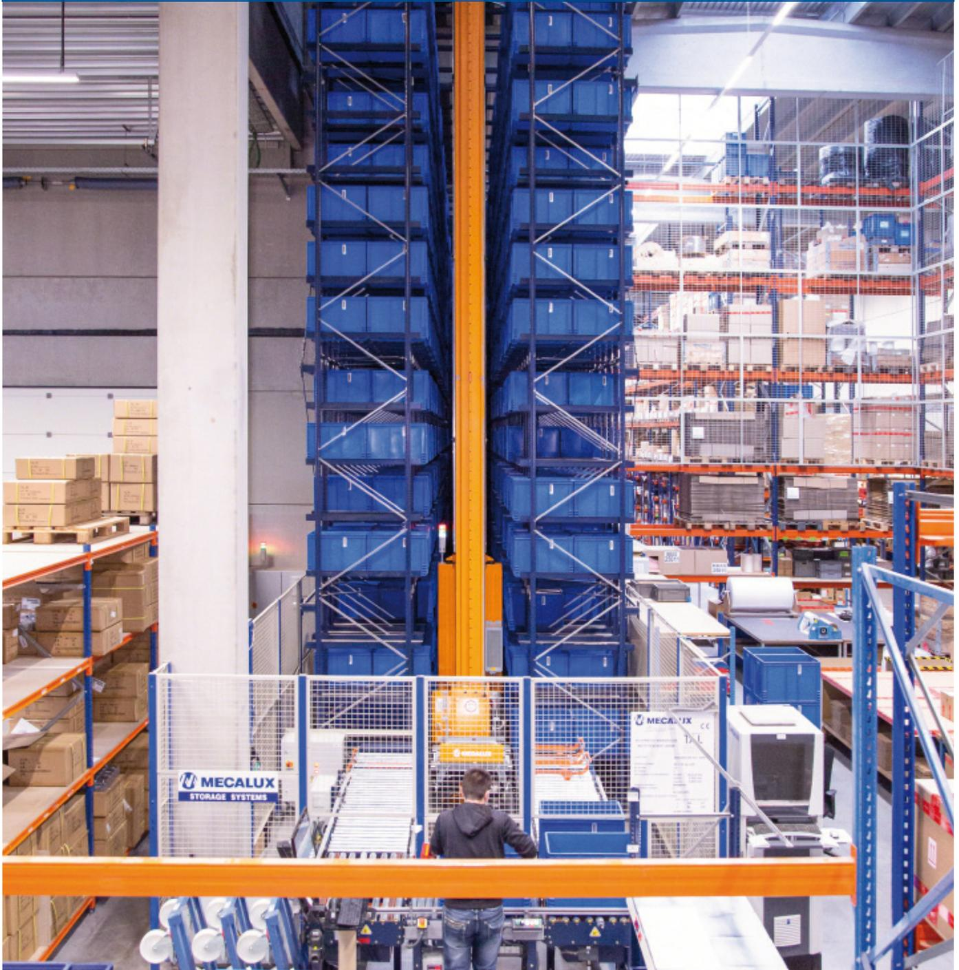
TAL, a Belgian manufacturer of high-quality lighting systems and accessories, has equipped its new distribution centre in Pittem, Belgium, with an automated warehouse for boxes. Its aim is to optimise space, ensure safe goods storage and minimise errors, ensuring the productivity required by omnichannel retail. Managed by Easy WMS, the facility holds approximately 1,400 SKUs in 6,300 boxes. Mecalux has also installed pallet and cantilever racks to store larger products.
