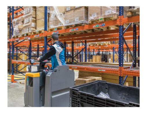
ing shelves. In total, this area stores 13,809 pallets containing goods of three different heights: 2.4 m, 1.9 m and 0.9 m. Therefore, pallet racks were the most suitable choice for storing pallets with many SKUs
