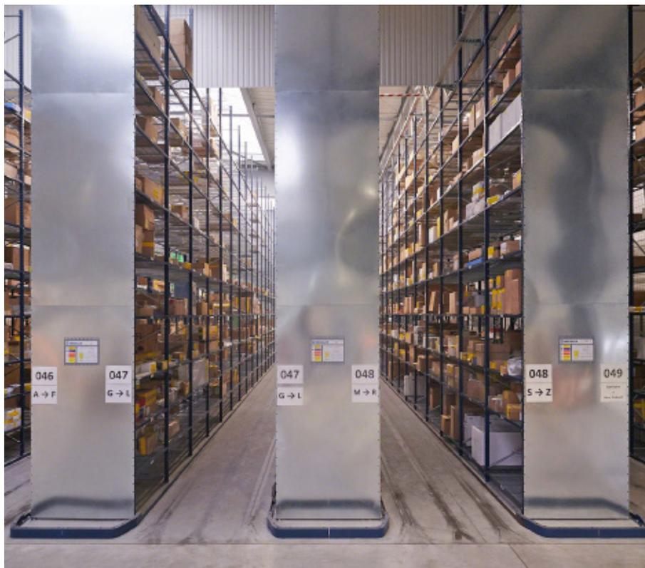
tre in Les Essarts. This facility serves the 750 members that form part of the cooperative. With the installation of two storage systems in one space, the company has achieved its goal. Movirack mobile racking is the only compact system that provides direct access to the goods in addition to optimising the surface area
