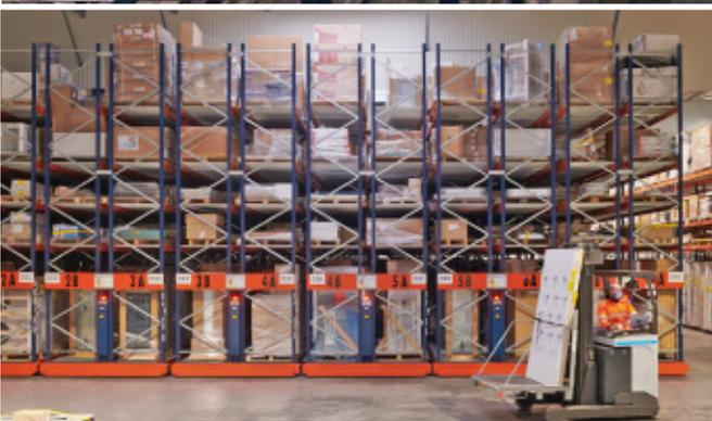
Cooperative VST has expanded its logistics centre in Les Essarts, France, and Mecalux has equipped it with Movirack mobile racking and multi-tier picking shelves. They have capacity for over 13,000 containers, which are stored according to their physical characteristics and weight. With this combination of solutions, VST has optimised its available space, sped up order preparation and reached its goal to dispatch more than 200 orders a day.
