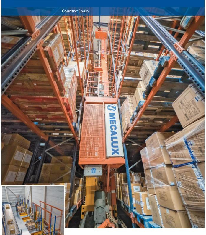
Gioseppo's facility in Elche (Spain) is composed of an automated clad-rack warehouse for pallets, with live racks and a specific area for picking. The warehouse management system Mecalux Easy WMS was supplied, which is responsible for managing all the centre's processes.
