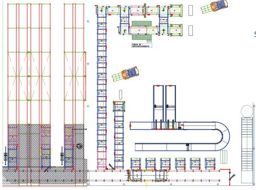
The picking area has six independent stations that are set up with a lift tables to improve ergonomic design
