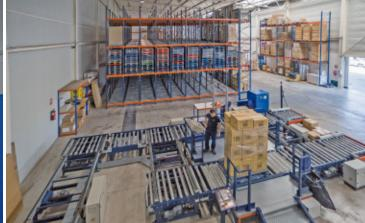
**Inputs and outputs**The inputs and outputs of palletised goods are done via a double shuttle that connects the main circuit of conveyors with the storage aisles. The goods input area has an entry checkpoint, which is responsible for verifying that the size, weight, and condition of the pallets comply with the facility's specifications.
