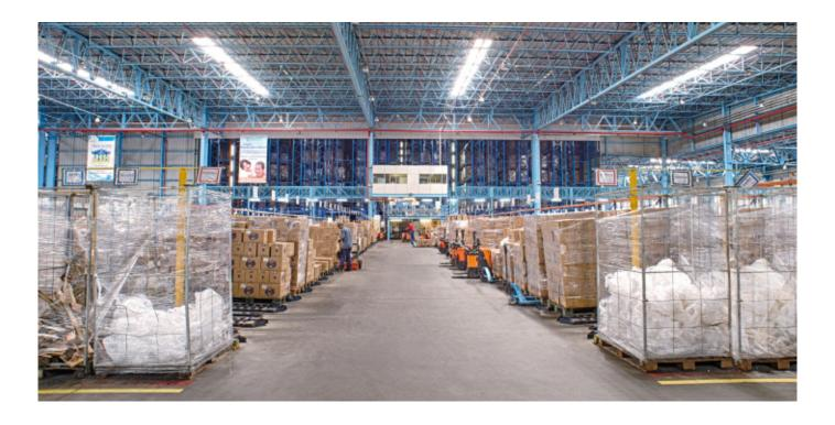
Ypê's facility in São Paulo, with a 24,168 pallet capacity, is expected to achieve a total flow of 200 pallets/hour in inputs and outputs Each grouping contains 66 channels with a three pallet capacity. The feeding is performed via transfer cars that automatically move from specific positions of the header to the live channels. The slight tilt with which channels are mounted allows the pallet to move by gravity to the closest free position in work aisles.
