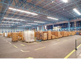
The input of the pallets that go into the warehouse takes place via three stations readied with a gauge control and input checkpoint equipment. This space is located in the reception dock area for incoming goods, occupying one of the sides of the warehouse.
