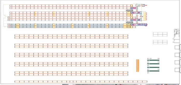
Incoming and outgoing processes in the warehouse are performed using a conveyor circuit that incorporates a pallet checkpoint. This checkpoint is used to check that the dimensions, weight and condition of the pallet meet the specifications of the installation.
