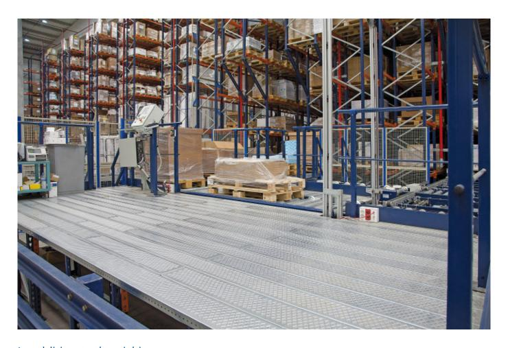
In addition to the picking station installed at the front, 44 live pallet channels have been enabled on the ground level
