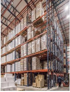
Built-in safety devices, like internal and external barriers with sensors, on the 12.3 m tall Movirack pallet racks keep personnel safe and guarantee the warehouse operates properly
