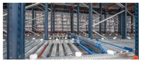
The live rack channels incline at a 4% angle, facilitating gravity flows of the pallets from the highest point (entries) to the lowest (exits)
