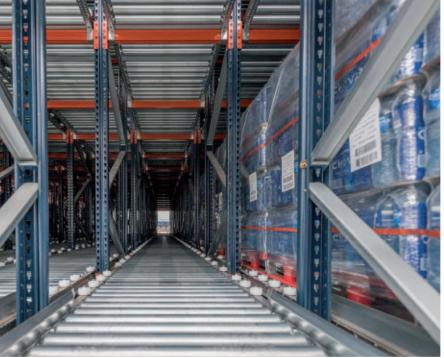
Mecalux has installed the highdensity Pallet Shuttle system and live racking in the water bottling plant of Manantiales del Portell, a company who focuses on collecting and bottling water under the brand Aguade Chóvar. The two warehouseing solutions represent a storage capacity that exceeds 4,600 pallets.
