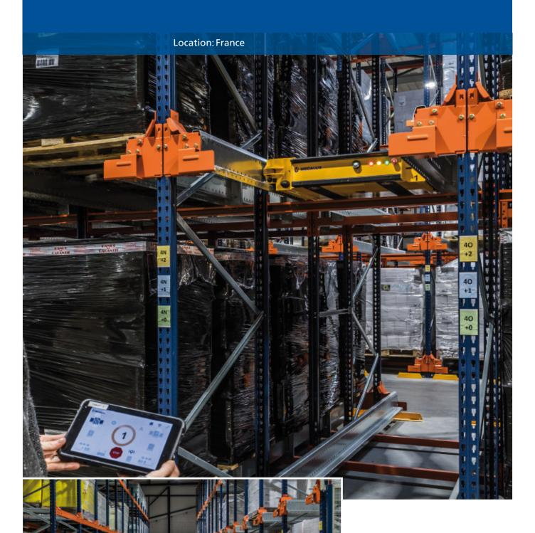
Vinaigrerie Générale has expanded its warehouse in Prigonrieux (France) with the objective of storing a larger number of SKUs. For this purpose, Mecalux has installed pallet racks, the Pallet Shuttle system and push-back racks which, altogether, offer capacity for 1,047 pallets.
