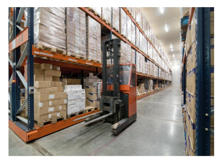
The mobile racking units are fitted with moving parts, electronic equipment and safety devices to protect the operators and the stored goods
