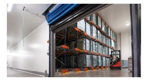
"The Pallet Shuttle's operation stands out for its simplicity," says Dan Bellaiche. The automatic shuttle moves the load to the first vacant position within the channel. While the Pallet Shuttle moves and deposits the pallet, the operator places another pallet in the first position of the same channel. That way, when the Pallet Shuttle returns to the front of the lane, it can repeat the same movement successively.
