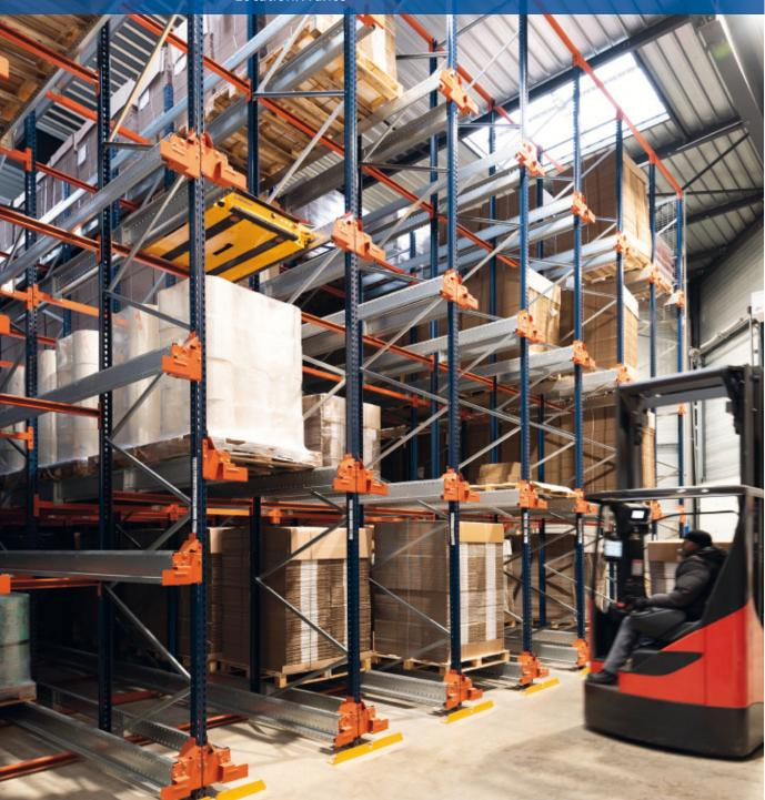
Les Mille Et Une Feuilles, which is a French puff-pastry maker (thus, the name 'a Thousand and One Leaves' in English), has opened a new warehouse with high-density racking and the Mecalux Pallet Shuttle system. This installation serves a dual purpose: to send raw materials to production and to store finished products. The Pallet Shuttle, being a semi-automatic solution, provides very fast inputs and outputs of the products.
