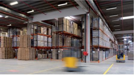
Pallet racks are one of the most widely used storage solutions employed by logistics operators in their distribution centres. The reason is obvious: these companies manage numerous customers and unit loads of varying sizes, and these racks easily adapt to their dimensions, characteristics and variable turnover. The new Dometrans warehouse in Templemars, northern France, houses 4,060 pallets containing packaging material for various customers.
