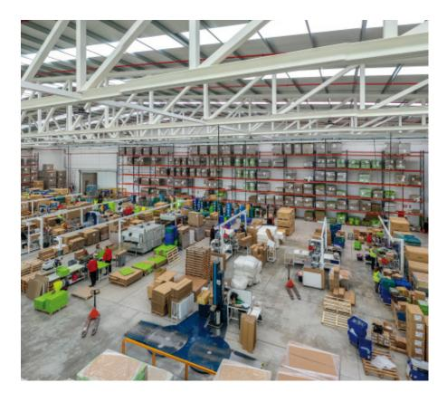
the storage area has been leveraged by narrowing the working aisles to the fullest extent. This has enabled the firm to maximise storage capacity in the smallest possible area. Francisco Martínez Piedras can store 6,606 pallets and access them all directly, thus facilitating goods flows and order prep.
