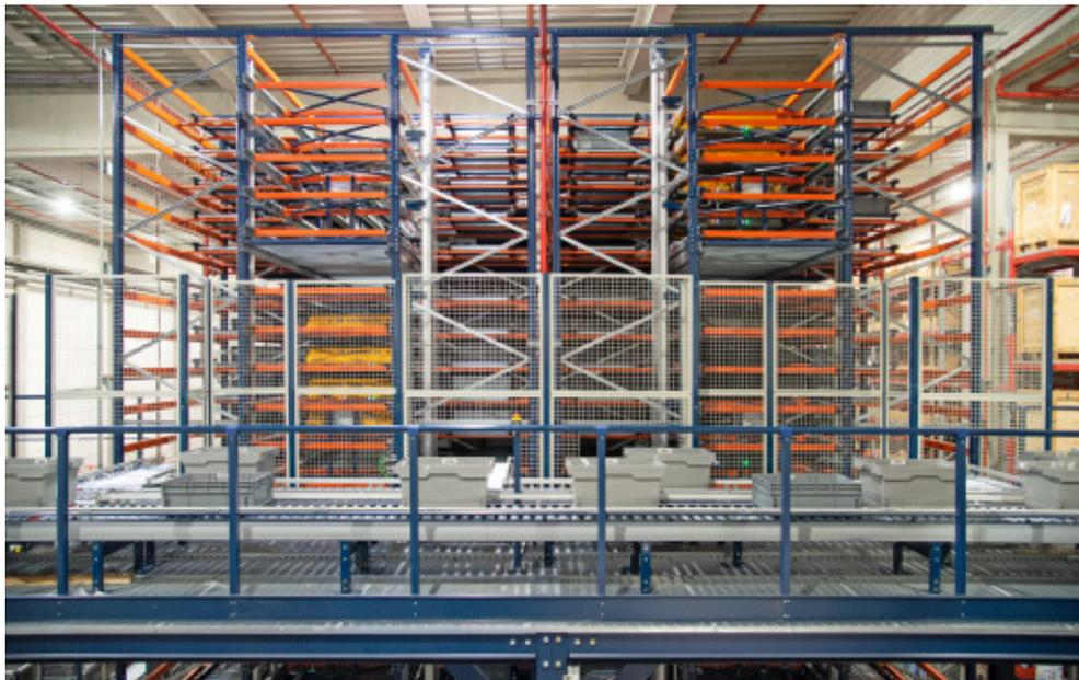
speeds up order picking. This solution provides a constant flow of goods from the storage area to the two high-performance pick stations.
